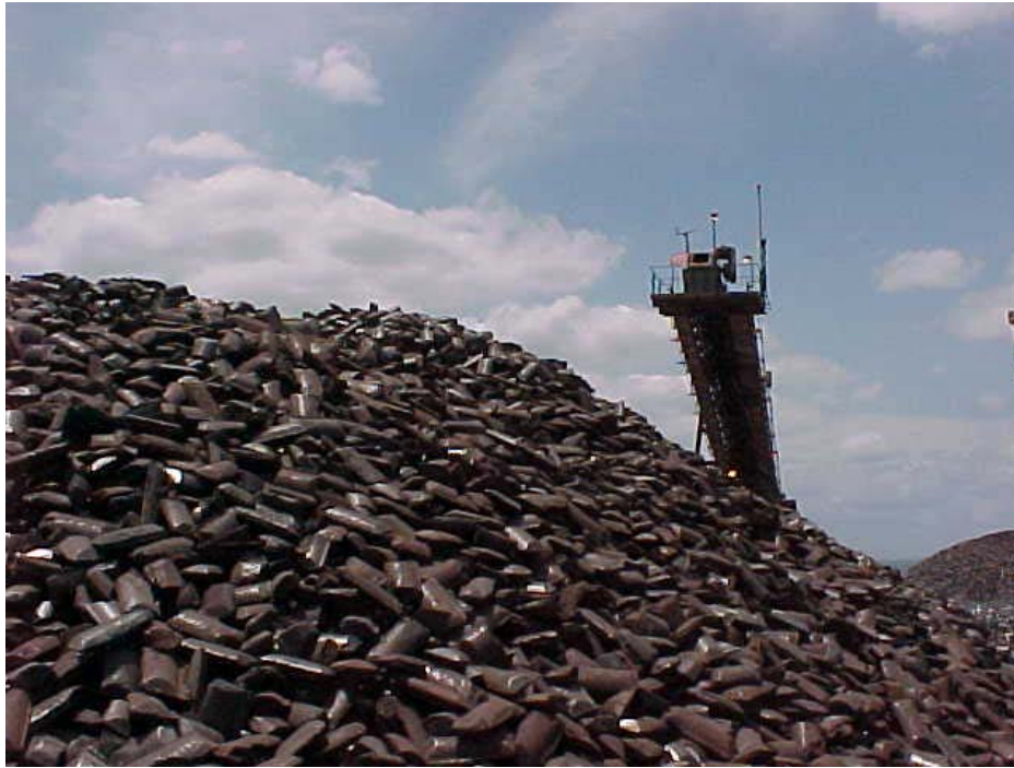
Exhibit 7 Output from the Briquetting Machine (HBI)
